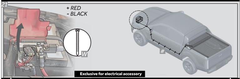
Do not pass the electrical harness near of moving parts or parts with large temperature variation.
