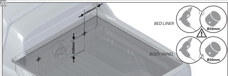
If necessary, remove the bed protector to clean any metal remains that could cause corrosion. Seal off areas with potential for water or dust ingress.
