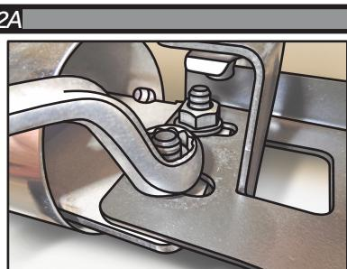
Release the two nuts, with french bolts, that hold the internal structure to the tube, so that you can adjust the tube with the "M" Right Base.
