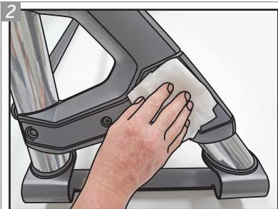
Clean the outer cover, in the area where the Side Plate will be placed, with isopropyl alcohol so that the glue has good adhesion.
